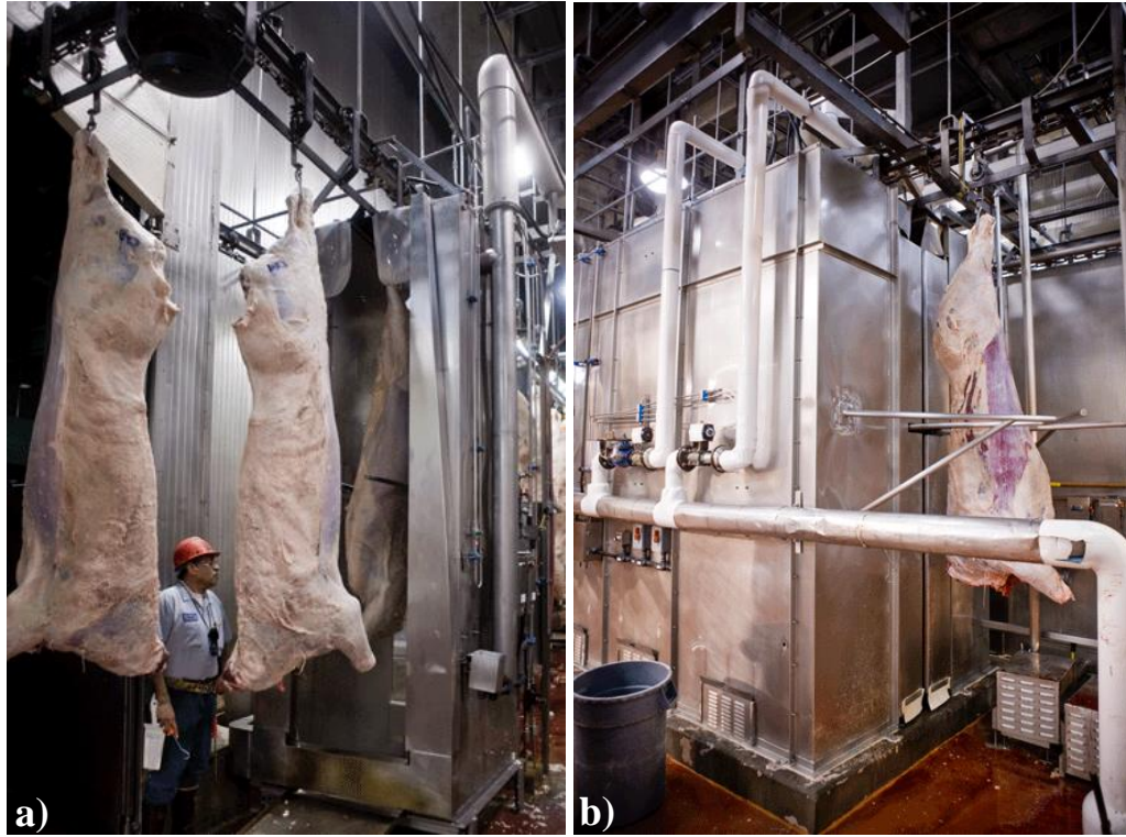
Figure 3.2: Examples of a) Organic acid spraying cabinet and b) Thermal pasteurization cabinet (Gabbett 2009)
